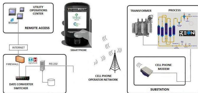
Fig. 3. Schematic diagram of the drying-out system data processing
