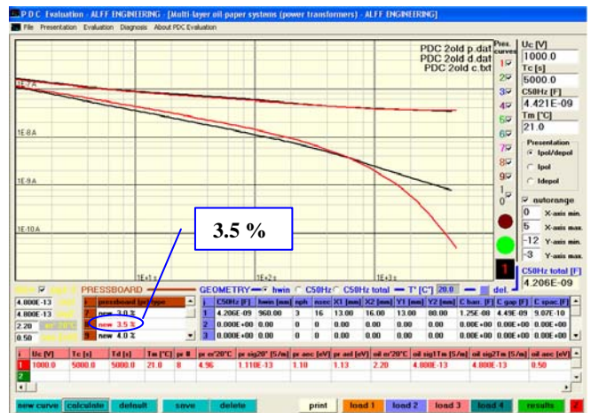
Fig.15. Moisture contents evaluation using PDC after 5 weeks running the molecular sieve drying-out system. Value 3.5 %.
