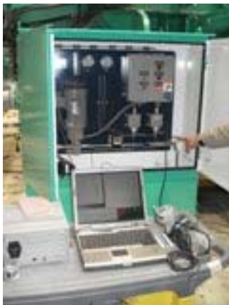
Figure 13. Particle in oil counter passes a light beam through oil filled vessel, and indicates the number of particles that block the light beam. Histogram of particle size is provided by this counter, since it tallies the particles that fall within the range: 4 \mu m; 6 \mu m; 14 \mu m and 24 \mu m. The particle counter has not been equipped with the digital output signal compatible with RS 485 bus, and at this stage cannot be included in the wireless monitoring system.
