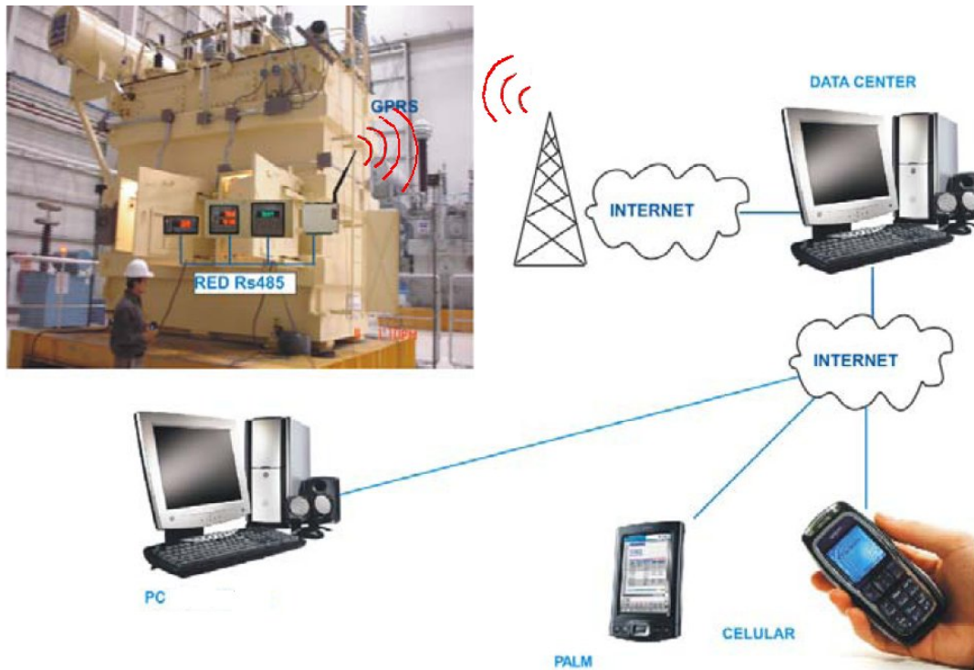
Figure 2. Schematic presentation of the wireless monitoring system. The sensors installed on the monitored transformer are of IED ( Intelligent Electronic Device ) type, and are directly connected to the short communication bus RS 485. Then, GSM ( Global System for Mobile Communication ) mobile-telephone transmitter sends them to the remote IDC ( Internet Data Center ) using GPRS ( General Packet Radio Service System ) protocol.
